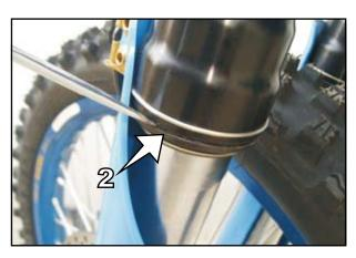
Clean the dust scraper, the outside legs and the rods carefully. Oil them well with silicone spray or with engine oil. Finally, push the dust scraper manually into the outside legs.
